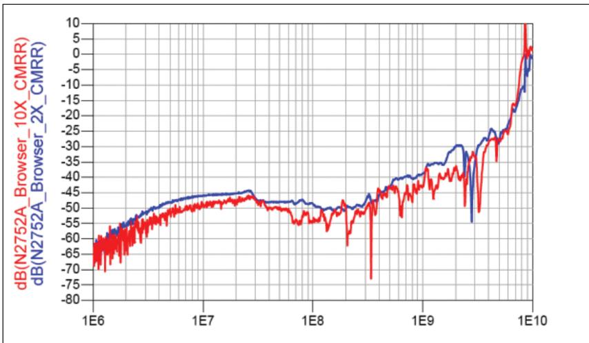
Figure 9. Common mode rejection ratio of N2752A (red: 2:1, blue: 10:1)
