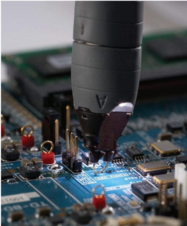
Figure 2. N2750A Series differential probe with browser tip
