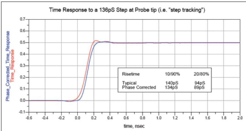
Figure 7. Time domain response to a 136 psec step of N2752A (at 2:1) with browser tip
