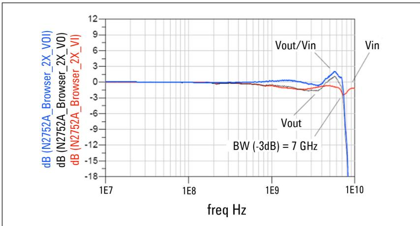
Figure 5. Vout/Vin frequency response of N2752A (at 2:1) with browser tip
