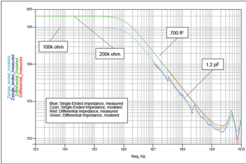
Figure 8. Input impedance over frequency of N2752A
